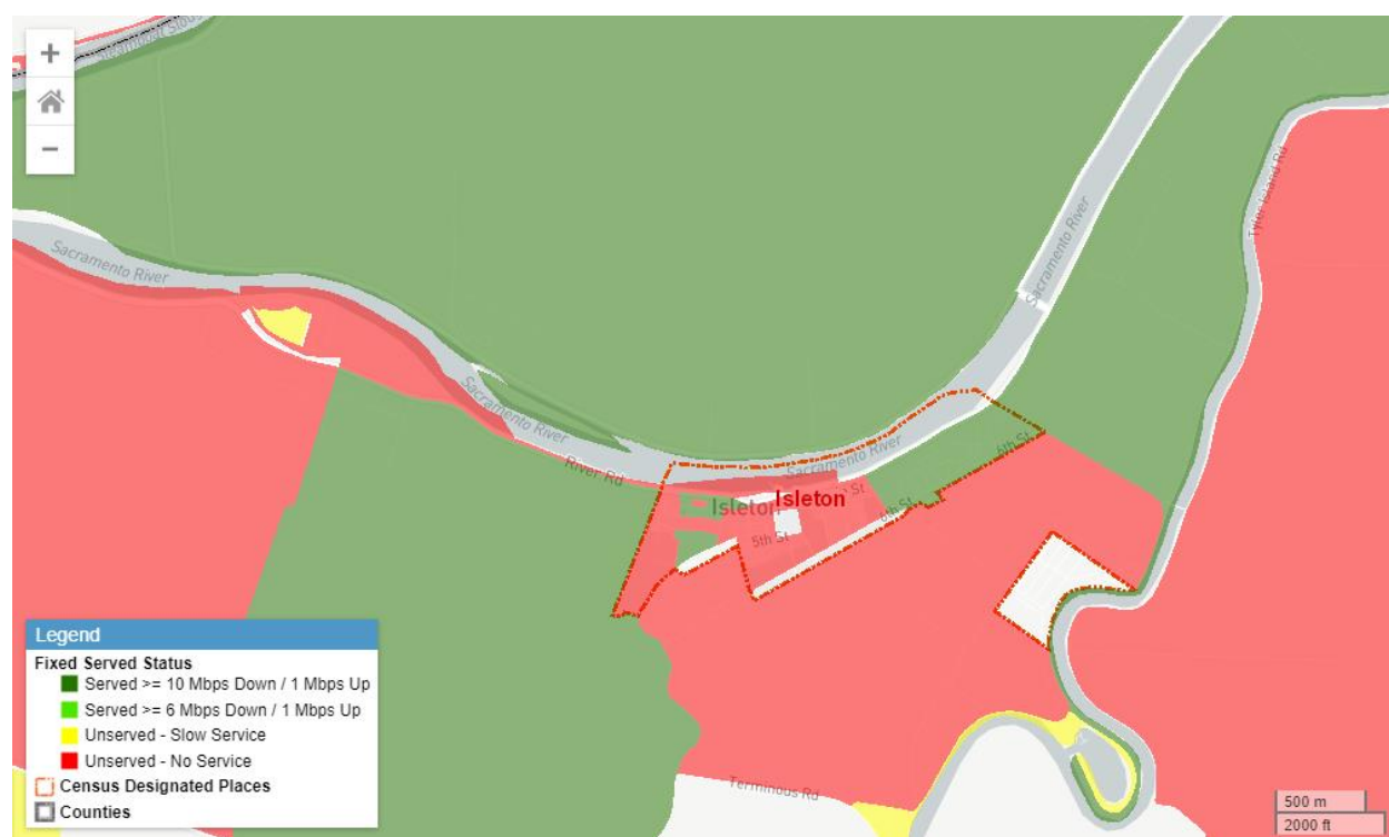
Figure 25. Aggregated fixed broadband service coverage in Isleton. Fixed broadband include both wireline and fixed wireless technologies. Green areas show coverage at or above the California broadband standard (6Mbps downstream and 1Mbps upstream) and darker green areas show coverage at or above 10Mbps downstream and 1Mbps upstream. Green and darker green areas might overlap as might be served at both speeds. Yellow areas show coverage at speeds below the California standard, and red areas show no internet service available.
